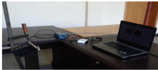
FIGURE 7: Vibration test setup with accelerometer attachment.
