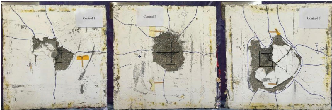
FIGURE 5: Control samples' failure modes.
