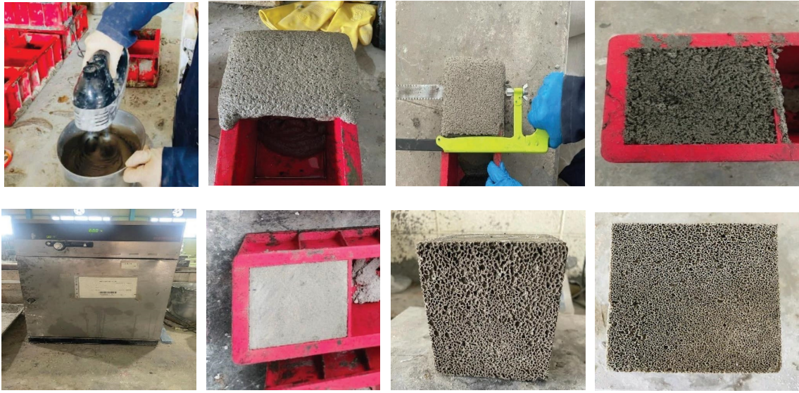
FIGURE 1: Geopolymer concrete cube production stages in order (mixing, molding, cutting, sample surface, curing, and final product).
