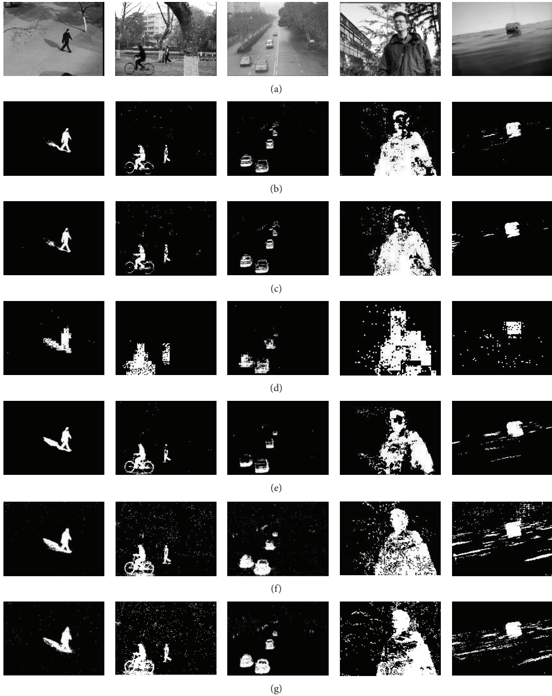
FIGURE 3: Comparative foreground masks of six methods. (a) Original frames, (b) our method, (c) ARCS, (d) CS-MoG, (e) ViBe, (f) KDE, and (g) GMM.
