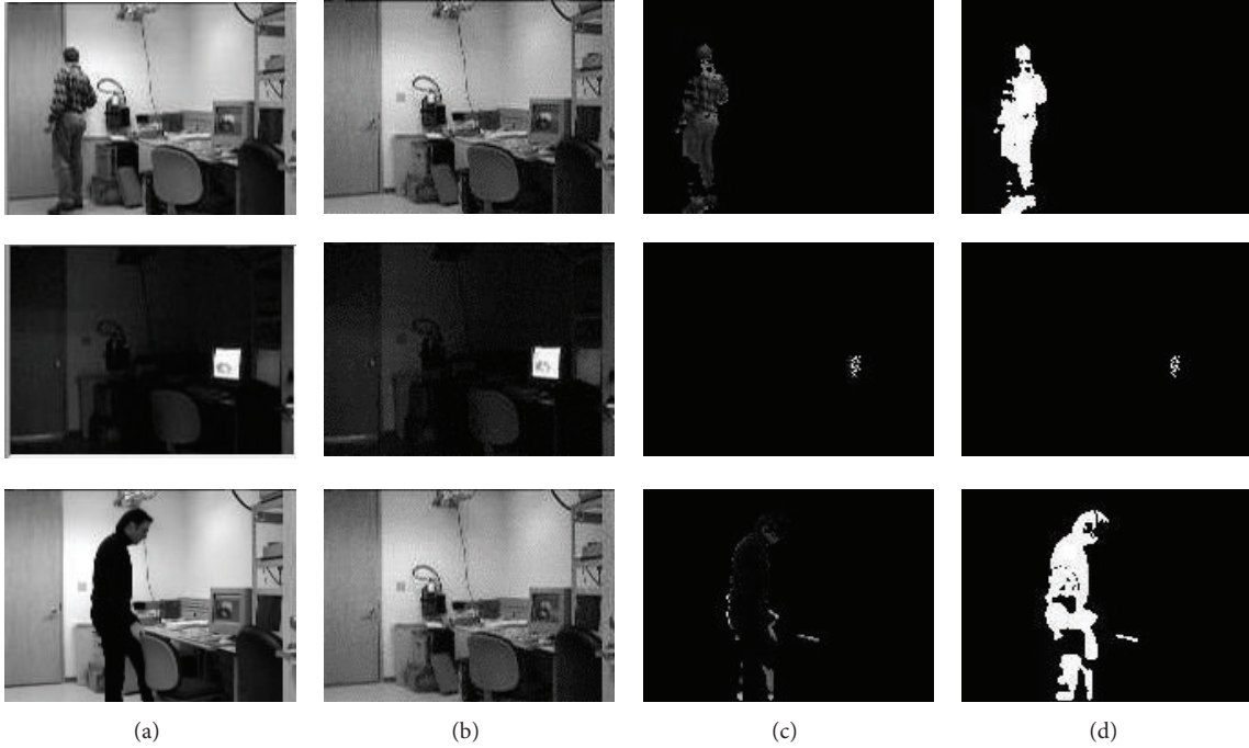
FIGURE 2: Results on a video sequence of 750 frames with sudden illumination changes. (a) Original frames, (b) background, (c) background subtracted images, and (d) foreground masks.
