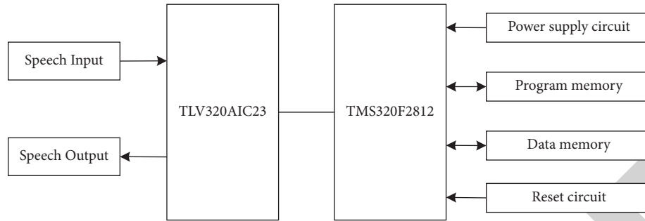
FIGURE 6: DSP speech enhancement system hardware structure design.
