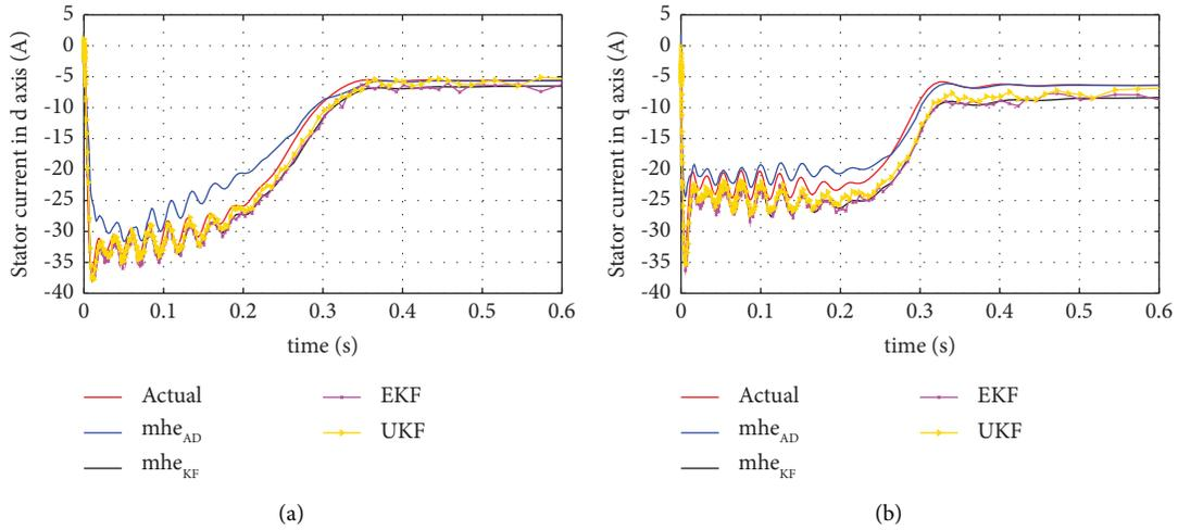
FIGURE 1: (a) Estimation of stator current in d axis. (b) Estimation of stator current in q axis.
