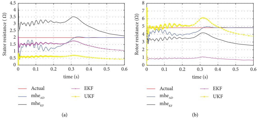
FIGURE 4: (a) Estimation of stator resistance. (b) Estimation of rotor resistance.
