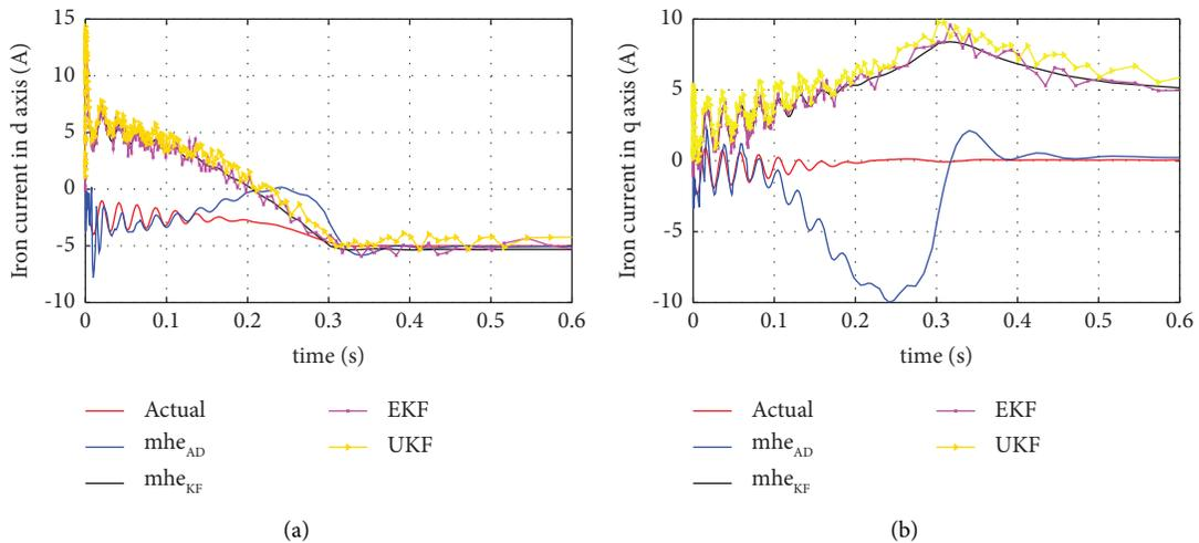
FIGURE 3: (a) Estimation of iron current in d axis. (b) Estimation of iron current in q axis.
