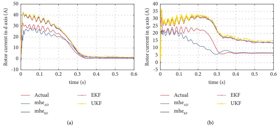
FIGURE 2: (a) Estimation of rotor current in d axis. (b) Estimation of rotor current in q axis.
