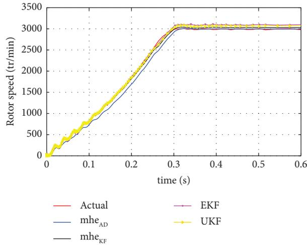
FIGURE 5: Estimation of rotor speed.
