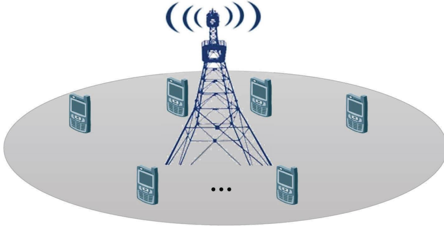
FIGURE 1: The system of a single-cell massive MIMO.
