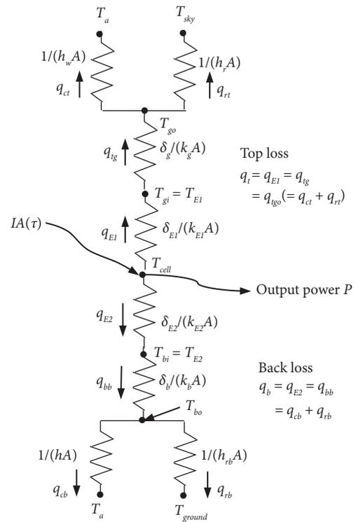
FIGURE 3: Thermal network for top and back losses of a solar PV panel.
