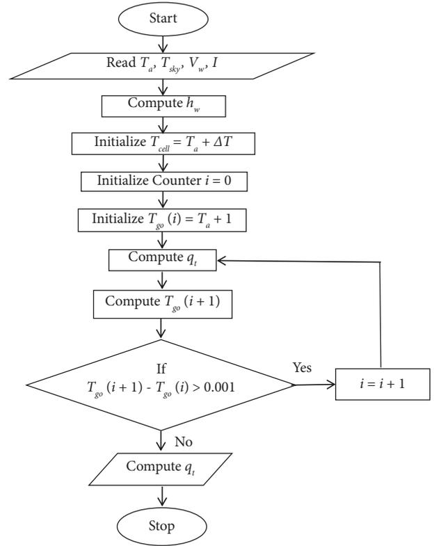
FIGURE 4: Flowchart for estimation of top loss.
