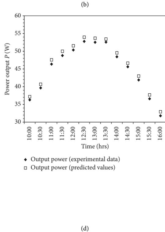
FIGURE 9: (a, b) Environmental parameters  $T_a$ ,  $I$ ,  $V_w$ , and  $T_{sky}$ , (c) panel surface temperatures, and (d) power output (predicted and experimental) versus time of the day (June 25, 2022).
