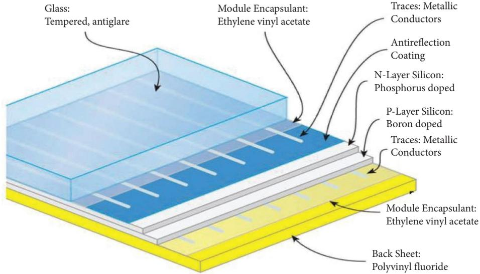
FIGURE 1: Basic construction of a solar PV panel [29].
