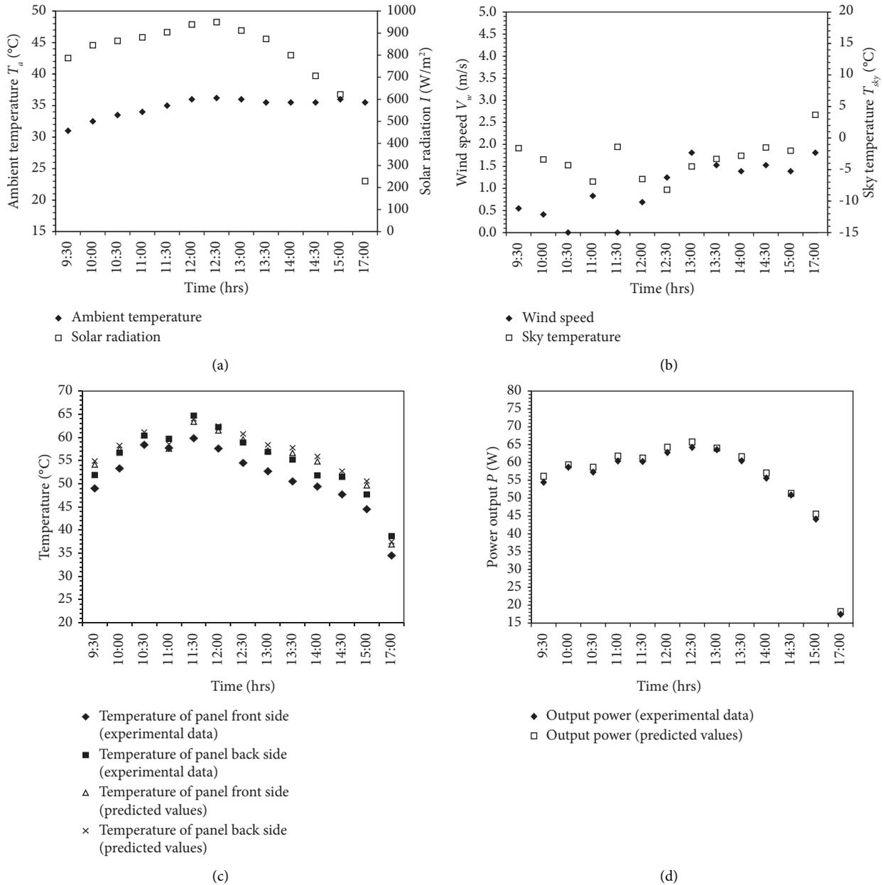
FIGURE 8: (a, b) Environmental parameters  $T_a$ ,  $I$ ,  $V_w$ , and  $T_{sky}$ , (c) panel surface temperatures, and (d) power output (predicted and experimental) versus time of the day (April 23, 2023).
