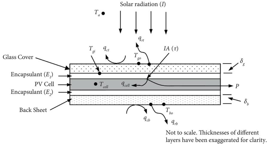
FIGURE 2: Energy balance on a solar PV panel.
