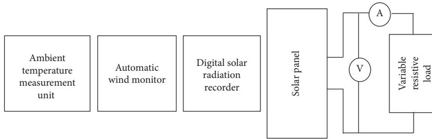
FIGURE 6: Schematic diagram of the experimental setup.
