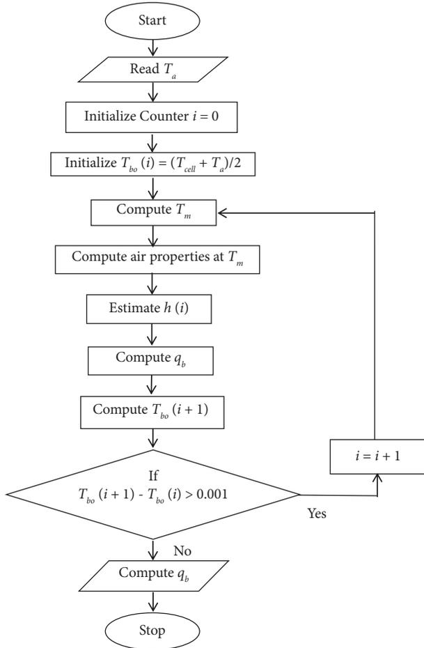
FIGURE 5: Flowchart for the estimation of back loss.
