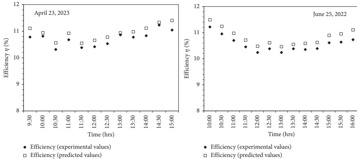
FIGURE 10: Predicted and experimental efficiency values versus time of the day.
