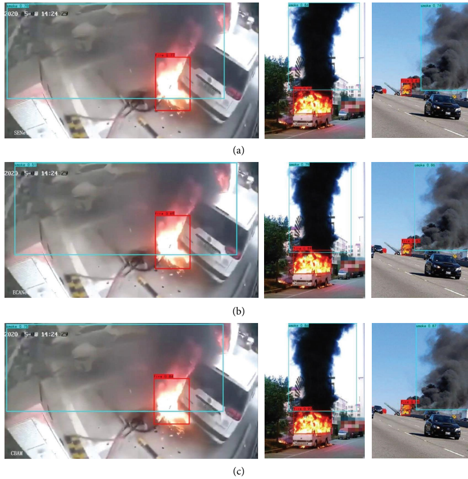
FIGURE 12: Comparison of picture detection results using SENet, ECANet and CBAM. (a) SENet. (b) ECANet. (c) CBAM.
