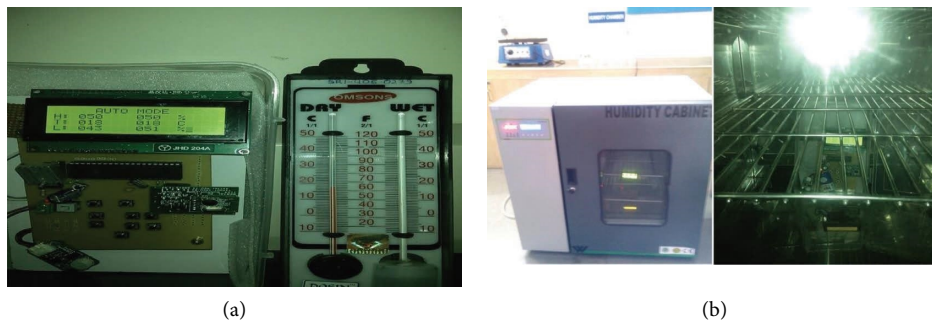
FIGURE 11: (a) Testing of a temperature sensor with a standard thermometer. (b) Testing of humidity sensor with a standard instrument.
