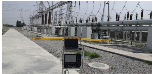
FIGURE 8: The UHF PD signal acquisition site.
