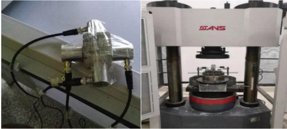
FIGURE 6: Placement of probes on loading specimens.
