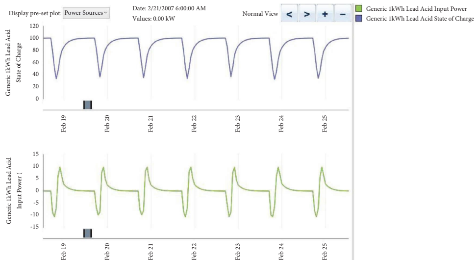
FIGURE 14: Hybrid system input power supplied to charge the battery and battery state of charge.
