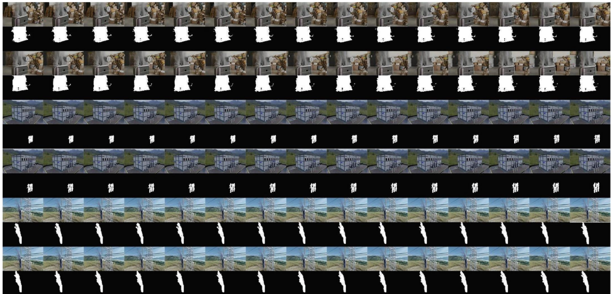
FIGURE 9: Segmentation effect of DS-UNet on continuous smoke images (two lines per scene).
