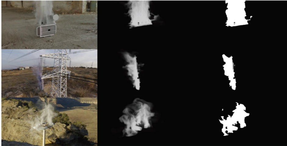
FIGURE 4: The smoke synthesis images and image masks generated by 3D virtual technology.
