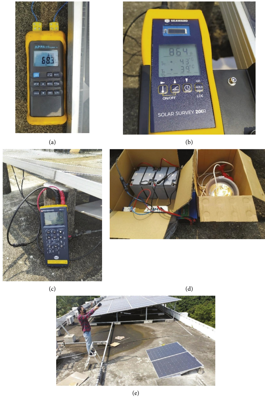
FIGURE 4: Data retrieval process and tools. (a) Solar module temperature using a contact thermometer, (b) irradiation value and ambient temperature using 200R solar survey, (c) IV curve data measurement, (d) simulated load installation on the system using battery and 500 W lamp, and (e) thermal image and visible light image collection FLIR camera.
