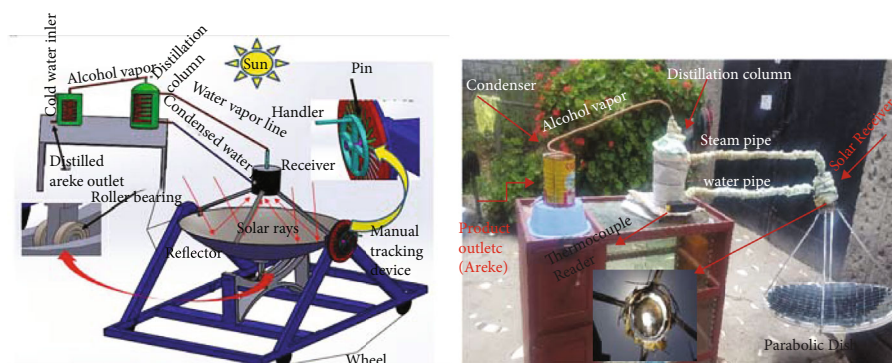
FIGURE 3: Schematic diagram (a) and experimental setup (b) of solar thermal local “Areke” Distillation system.
