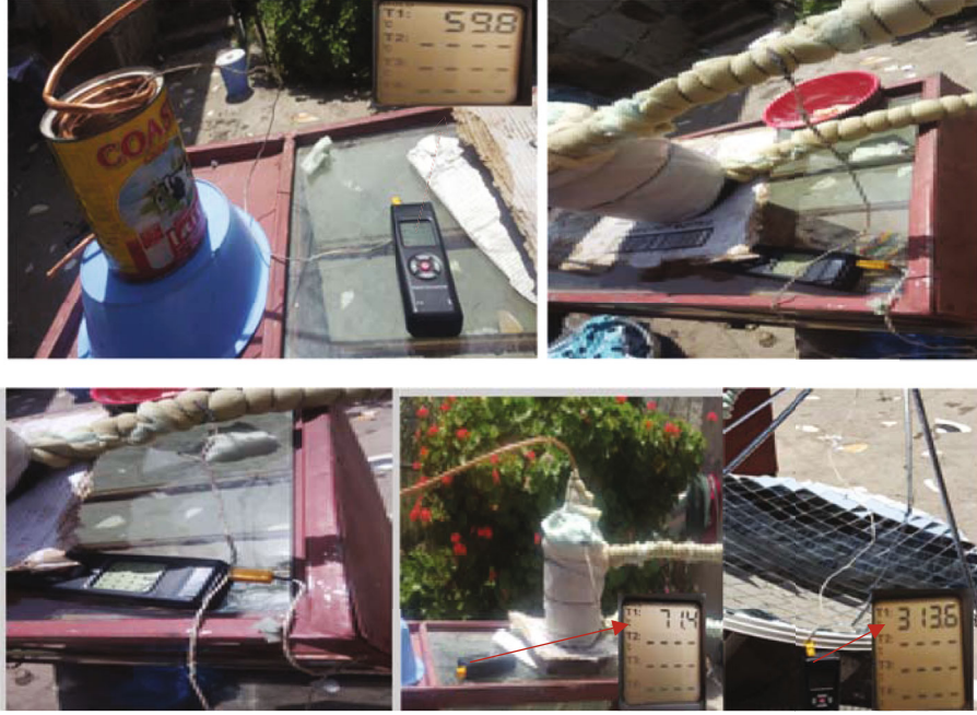
FIGURE 4: Installation position of the thermocouple.
