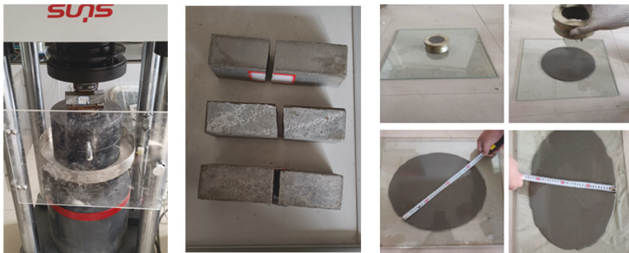
FIGURE 4: Grout properties test.
