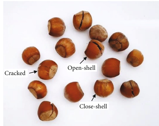
FIGURE 1: Samples obtained from the output of the hazelnut cracking machine.
