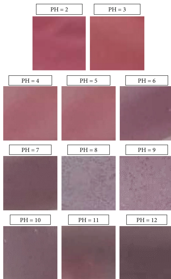
FIGURE 8: Color changes of the film containing 45% purple carrot extract at different pH.
