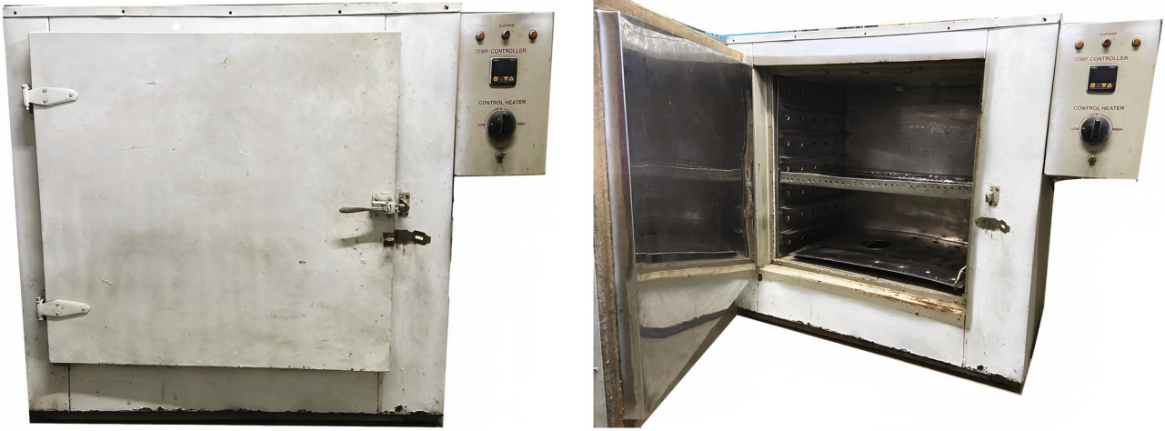
FIGURE 1: Photographic view of the laboratory cabinet dryer used for sweet potato drying.
