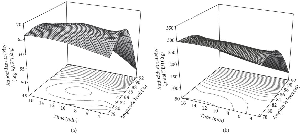
FIGURE 1: Effect of the ultrasound extraction on the antioxidant activity of green cactus pear seed oil. (a) ABTS; (b) DPPH.
