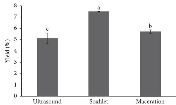
FIGURE 3: Cactus pear seed oil yield achieved by different extraction methods. <sup>a,b,c</sup>Different letters mean significant differences between methods ( $p < 0.05$ ).
