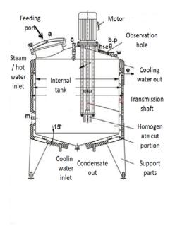
Supplementary Figure 1. The draft of the device used for homogenate extraction.
