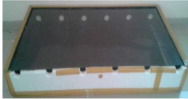
FIGURE 7: Solar dryer with thermocol insulation.
