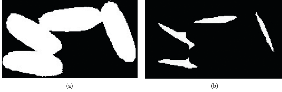
FIGURE 8: Baseline endpoint matching diagram. (a) The binary image. (b) The obtained seed image.
