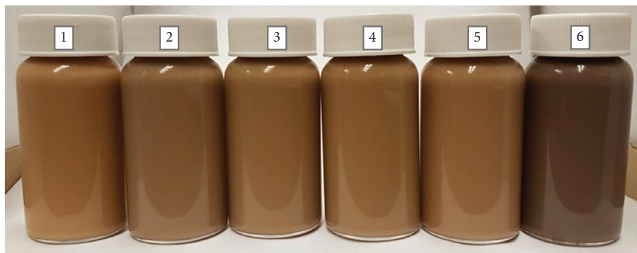
FIGURE 8: Indian-style milk tea brewed with iron microcapsules and EDTA (2–4), visual colour comparison with regular tea as a positive control (1), and unencapsulated iron as a negative control (6) as listed in Table 3.
