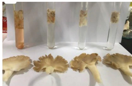
FIGURE 2: Effect of temperature on inactivation of PPO enzyme during blanching (control -60-70-80°C).
