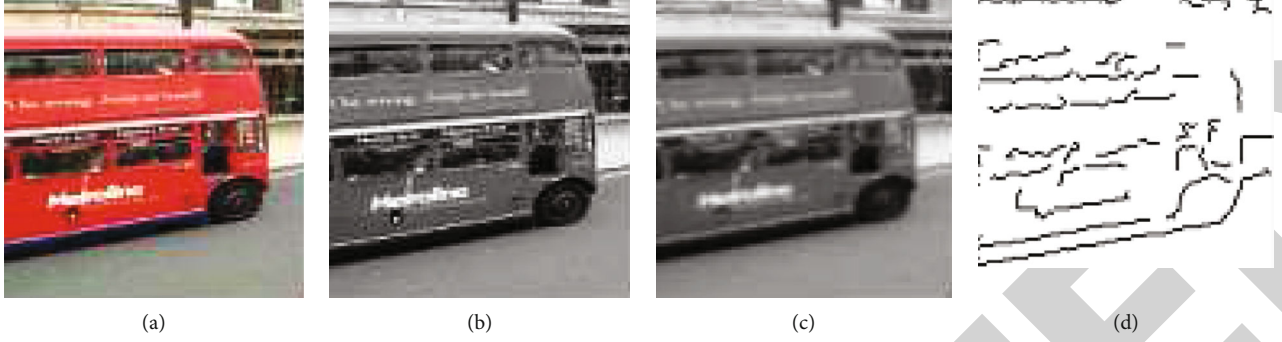
FIGURE 2: From raw image to edge detection: (a) Raw image, (b) image after grey-scale conversion, (c) blurring after median filtering, and (d) edges extracted from the image.
