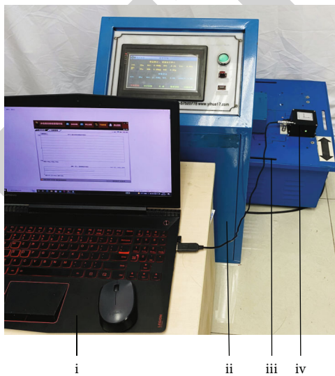
FIGURE 7: Function and performance test picture. (a) PC monitoring. (b) Vibration test console. (c) Vibration test platform. (d) Shock and vibration acceleration recorder.
