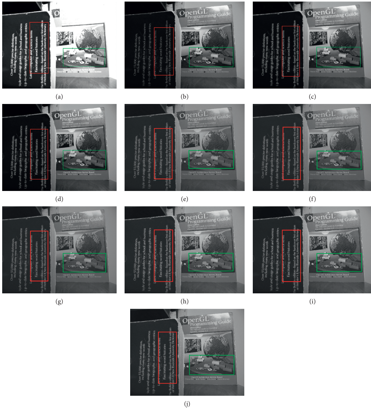
FIGURE 7: The fusion results of “books image set”: (a) average fused, (b) minimum fused, (c) DWT fused, (d) SWT fused, (e) DWT + LF fused, (f) DWT + UM, (g) DWT + (LF + DFT), (h) SWT + LF, (i) SWT + UM, and (j) SWT + (LF + DFT).
