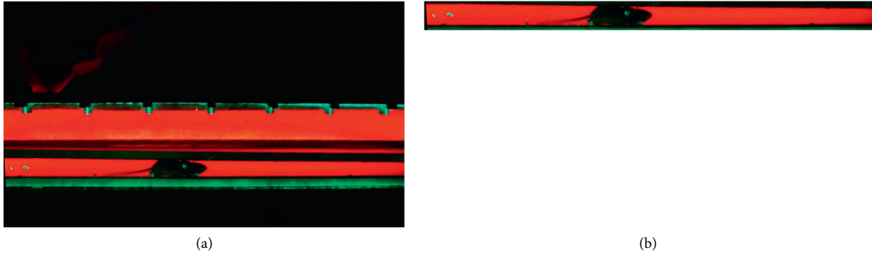
FIGURE 5: Application of the preprocessing steps to a sample image. (a) Image after correcting for rotation. (b) Cropped image showing just the glass trackway.
