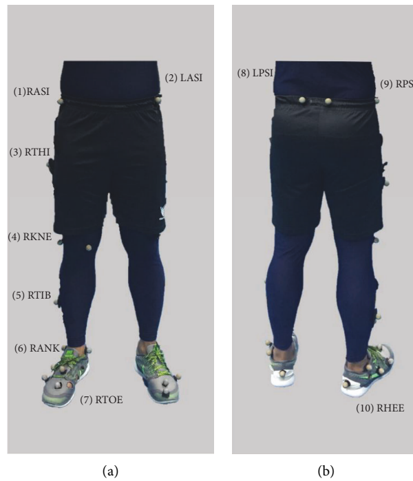
FIGURE 2: Marker's position on the subject's body in (a) front view; (b) rear view.
