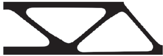
(a) Eroded design f = 290.009, volfrac = 0.5, \eta = 0.25
