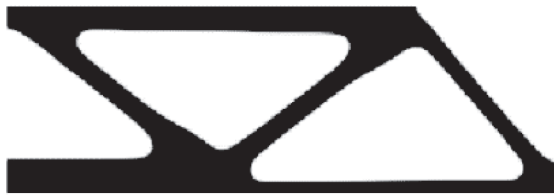
(a) Eroded design f = 270.821, volfrac = 0.5, \eta = 0.25
