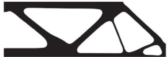
(a) Eroded design f = 260.614, volfrac = 0.5, \eta = 0.25
