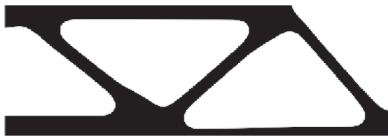
(a) Eroded design f = 303.678, volfrac = 0.5, \eta = 0.25
