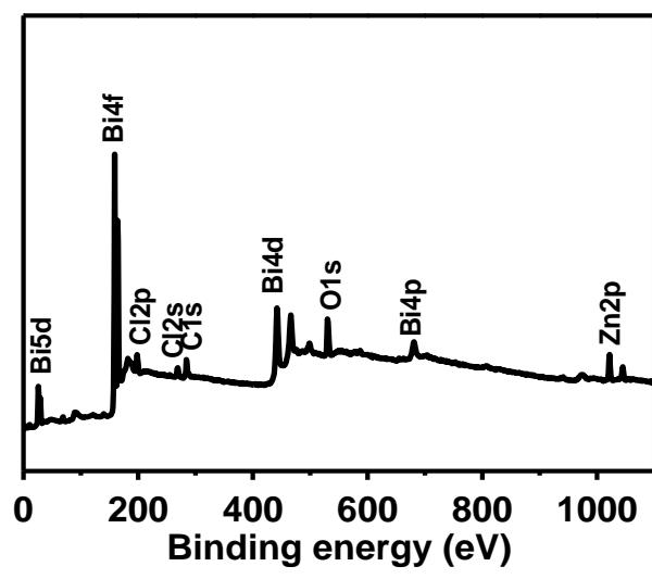
**Fig. S1.** XPS survey spectrum of the  $(\text{BiOCl})_{0.6}(\text{ZnO})_{0.4}$  composites.
