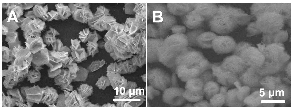
**Fig. S2.** SEM images of individual ZnO (A) and BiOCl (B)
