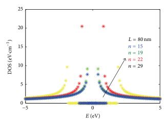
FIGURE 4: DOS versus E for various values of chirality (n) and L = 80 nm.
