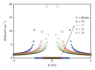
FIGURE 5: DOS versus E for various values of chirality (n) and L = 60 nm.
