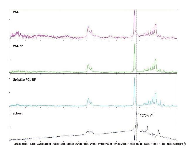
Supplementary material 2. FT-IR spectrum of component and samples of nanofiber. PCL, PCL
