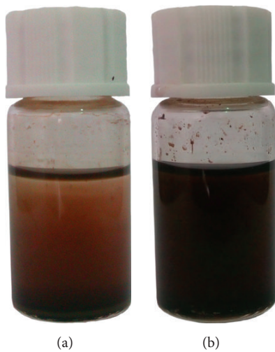
FIGURE 3: Dispersion state of MoS 2 nanosheets in base olefin after 24 h: (a) RM-MoS 2 and (b) DDT-MoS 2 .
