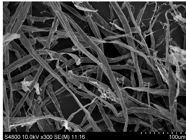
Figure S1: The morphology of original eucalyptus pulp fibers. The fiber dimensions were \geq 10 \mu\text{m} in diameter and \geq 200 \mu\text{m} in length.
