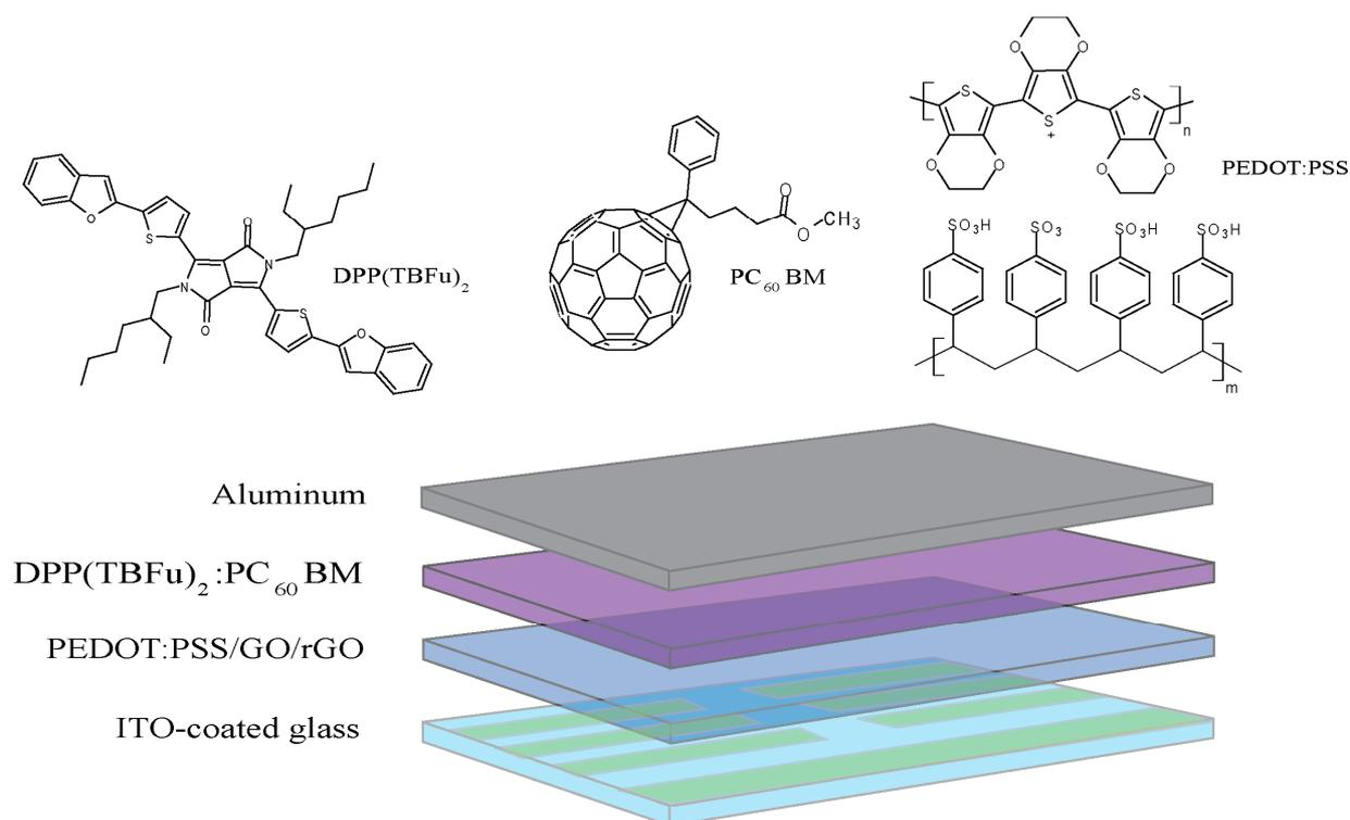
**Fig. S2:** The final structure of organic solar cells with bulk heterojunction
