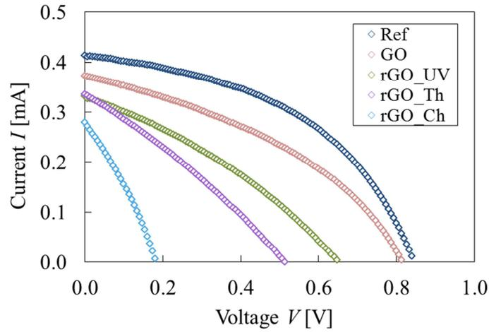
**Fig. S2.2:** The influence of hole-extraction GO layer and its reduction of I-V characteristics
