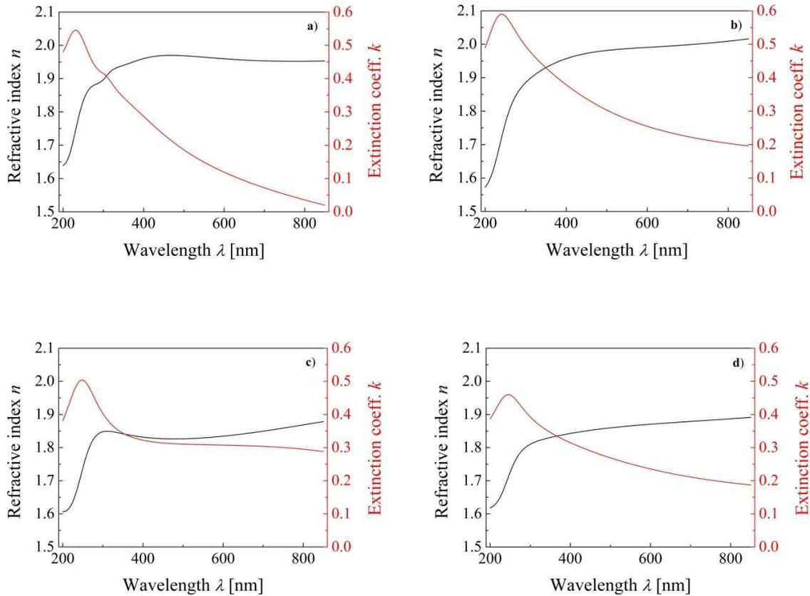
**Fig. S1:** Dependencies of refractive index and extinction coefficient spectra of a thin film: a) GO, b) the thermal reduced GO, c) the chemical reduced GO and d) UV reduced GO
