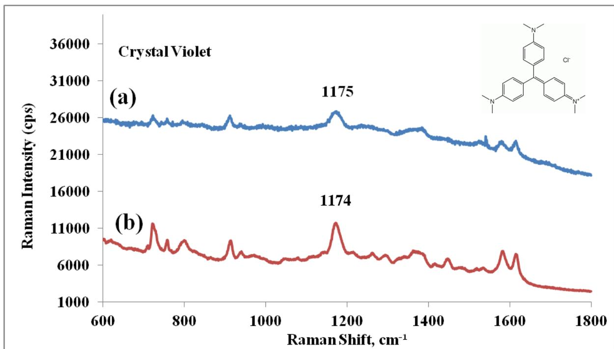
Fig. 3. Raman spectrum of solid CV(a) and SERS spectrum of  $10^{-5}$  mol/L CV dropcasted onto 60 nm AuNP@Al foil (b), taken with 633 nm excitation wavelength .
