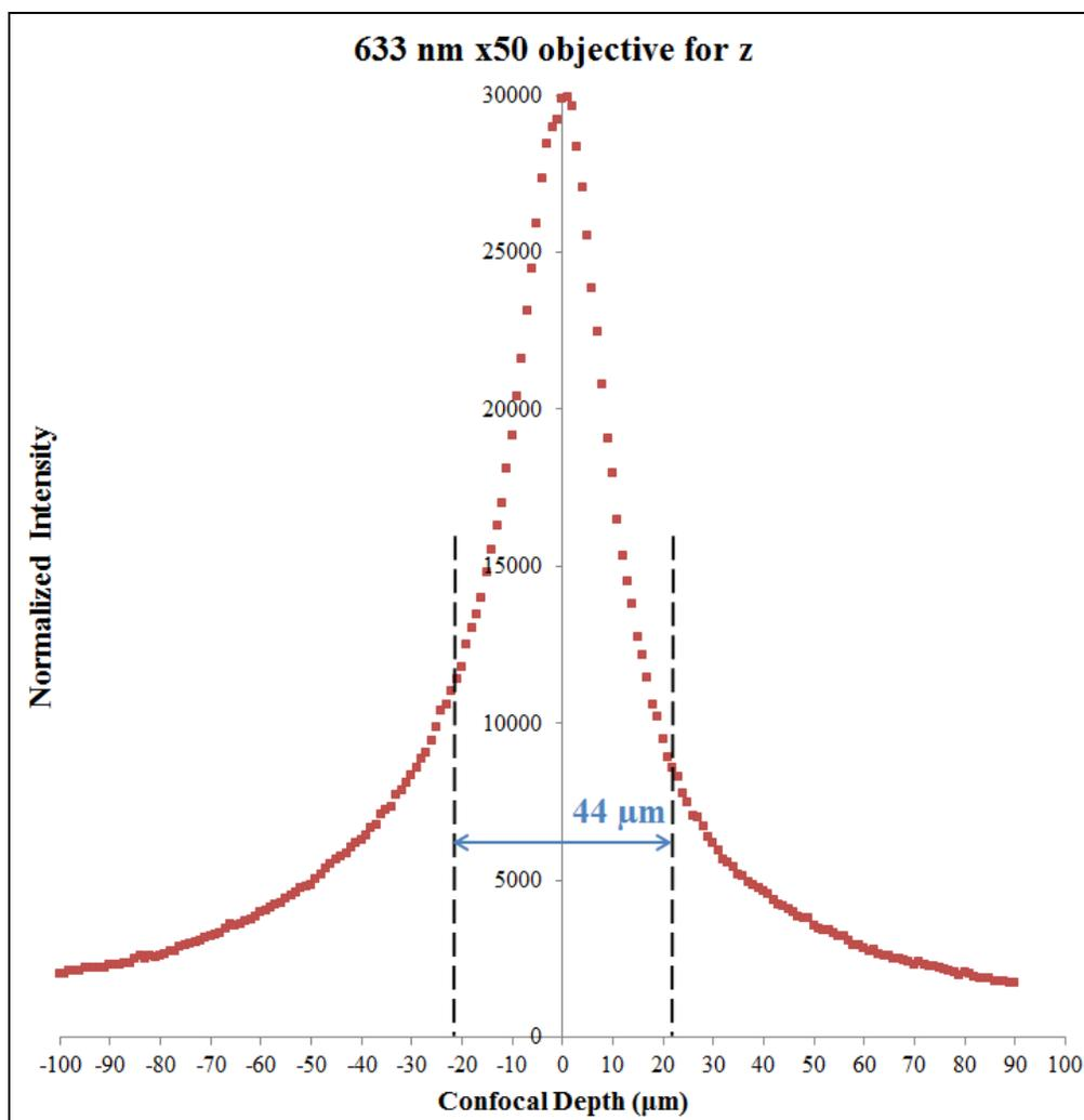
Fig. 7. Raman intensity(I) –confocal depth (z) profile of the normalized intensity of solid 4-NBT. SERS measurements were performed using 633 nm excitation from a He-Ne laser and a 50X objective
