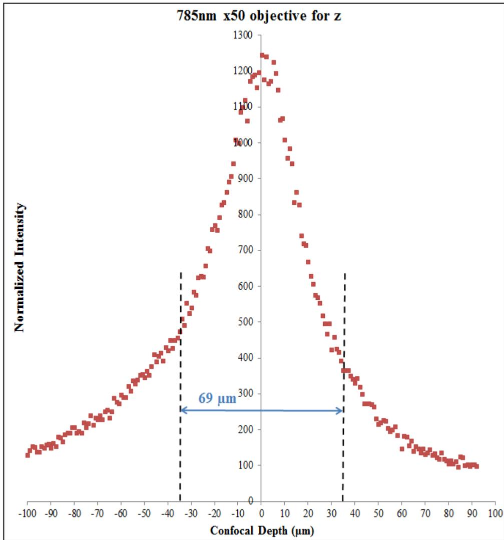
Fig. 6. Raman intensity (I) – confocal depth (z) profile of the normalized intensity of solid 4-NBT. SERS measurements are performed using 785 nm excitation from a He-Ne laser and a 50X long working-length objective.<sup>2</sup>
