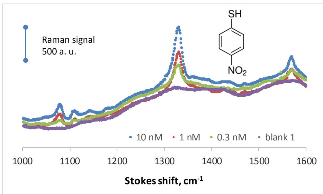
Figure 2. SERS spectra of NBT on 60 nm AuNPs @ Al foil at various concentrations of NBT, taken with 633 nm excitation wavelength.
