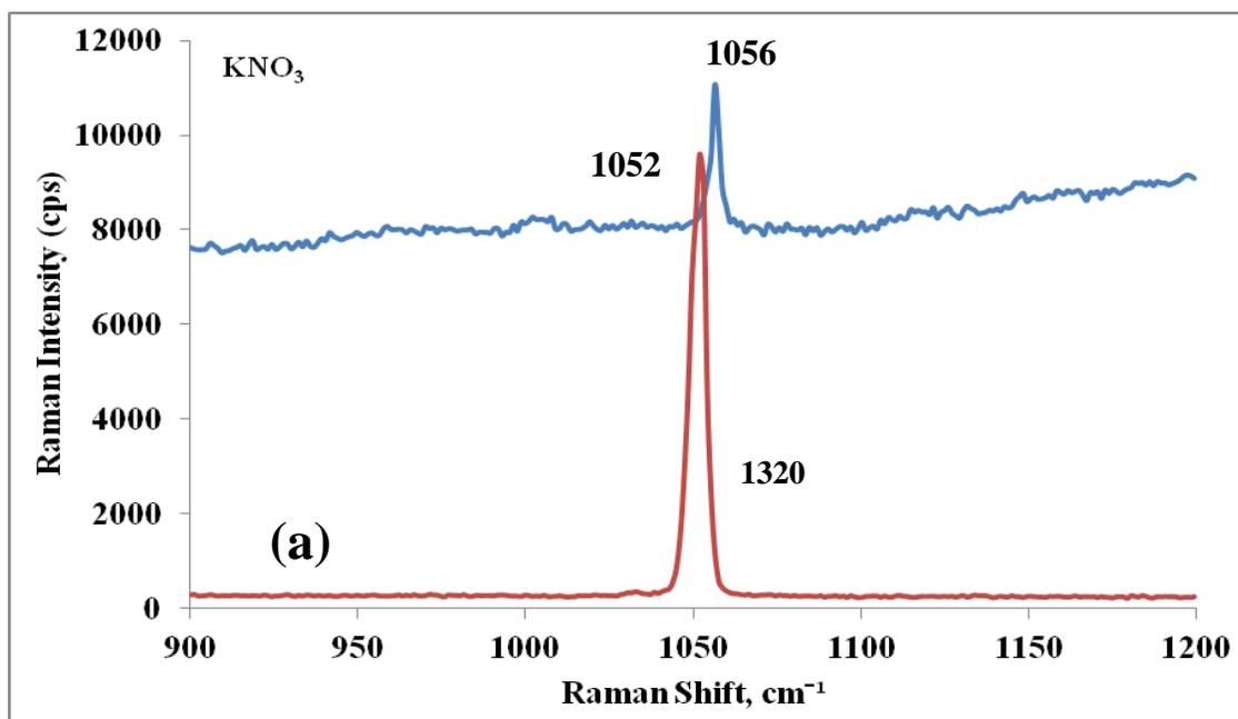
Fig. 4. Raman spectrum of solid  $\text{KNO}_3$  powder (a) and SERS spectrum of  $16 \times 10^{-3}$  mol/L  $\text{KNO}_3$  dropped onto 40 nm AuNP@Al foil (b), taken with 785 nm excitation wavelength.
