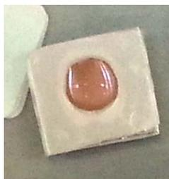
Fig1. AuNP solution dropped onto AuNP@Al foil.
