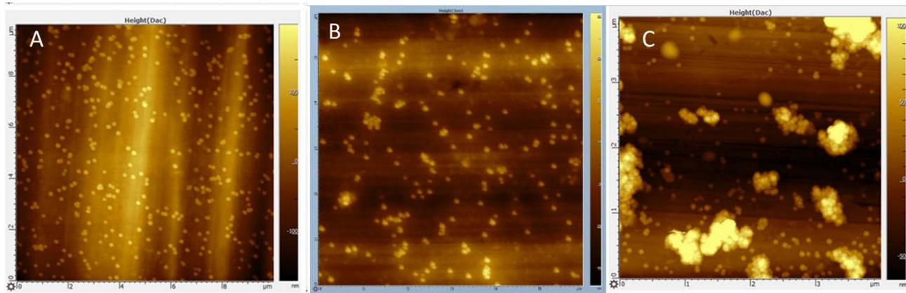
Fig.5. Unprocessed AFM images of AuNP@Al foil substrate: A) 60 nm AuNPs for CV, B) 60 nm AuNPs for NBT, C) 40 nm AuNPs for  $\text{KNO}_3$ .
