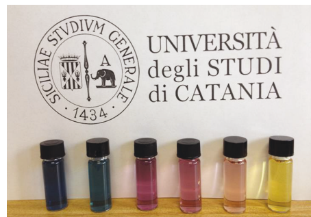
FIGURE 1: Some of the colloidal dispersions obtained. Different colors correspond to different plasmon resonance features.
