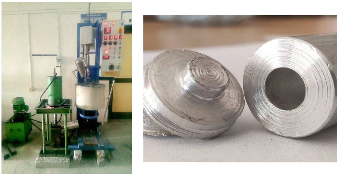
FIGURE 1: Squeeze casting setup and novel encapsulated metal cap.
