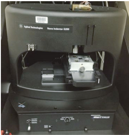
FIGURE 2: Agilent G200 nanoindenter and nanoscratch device.
