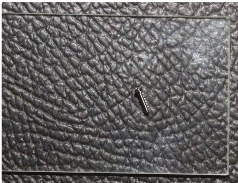
FIGURE 1: Photograph showing commercially pure self-tapping micro titanium osteosynthesis implant screws (4 mm × 2 mm).
