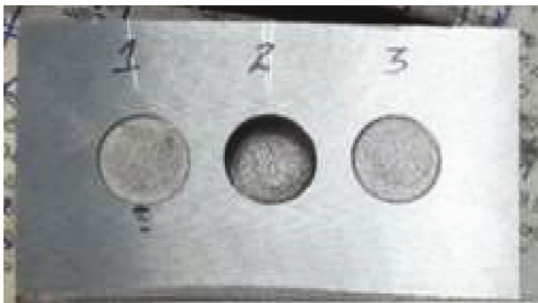
FIGURE 7: Illustration of SS630 grade workpiece after machining.
