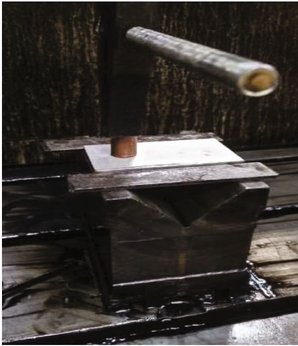
FIGURE 6: Machining procedure of DS-EDM.
