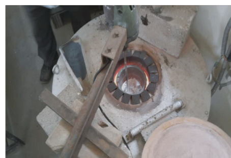
FIGURE 2: Molten metal is stirred in the furnace.
