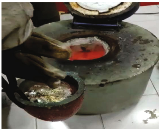
FIGURE 1: Stir casting fabrication setup.
