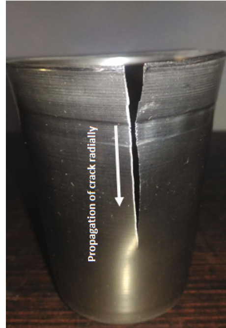
FIGURE 3: SSLNA radial propagation of crack.
