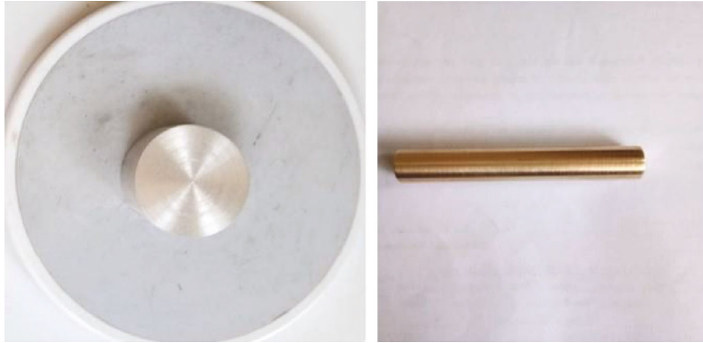
FIGURE 1: Prepared specimen of the workpiece (diameter 34 mm and thickness 10 mm) and tool electrode (diameter 10 mm).
