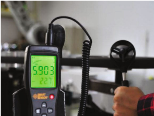
FIGURE 10: Cooling air flow velocity in the space near the processing area.
