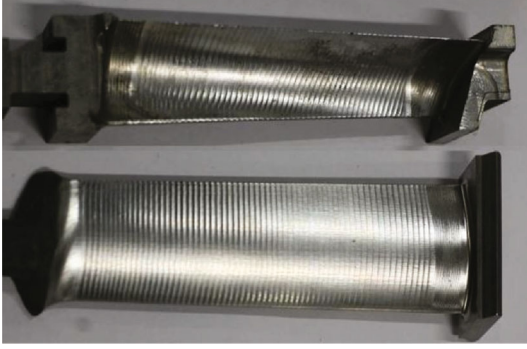
FIGURE 1: Blades formed by CNC milling.
