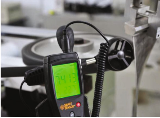
FIGURE 9: Cooling air flow velocity in the contact area during blade machining.
