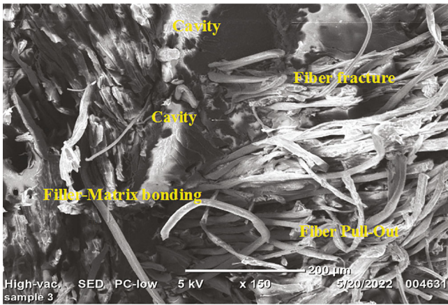
FIGURE 11: SEM image of the tensile-fractured surface for EBGCM2.
